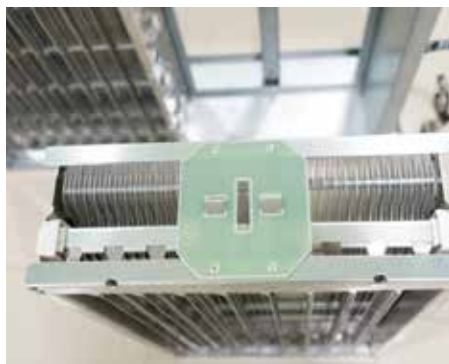
Step 2: load the bottom of the ion tank into the housing
