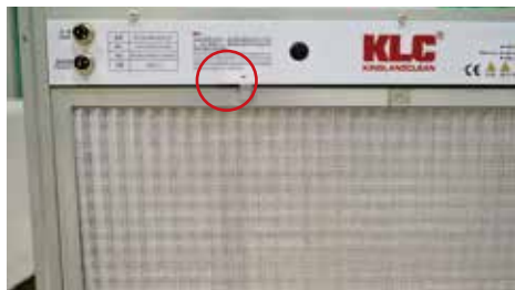
Step 1: Rotate the buckle
